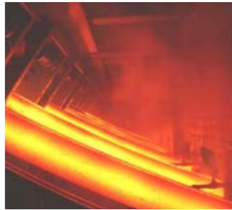
Billet feedstock Our rolling mill uses billet feedstock produced at the SMACC melting shop.
