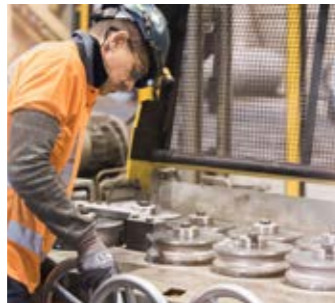
Cold drawing Wire rod is drawn through a die, reducing the cross-sectional area of the bar, and cut to lengths.
