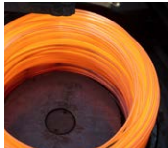
Wire rod coiling Wire rod of up to 10 mm is coiled on a laying a head. Rod in larger diameters is coiled in garrett coilers.
