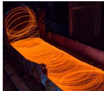
Coil forming Wire rod of up to 18 mm is coiled on a laying head.
