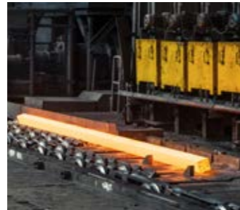
Reheating furnace Accurately controlled, two-stage reheating minimizes surface scaling.
