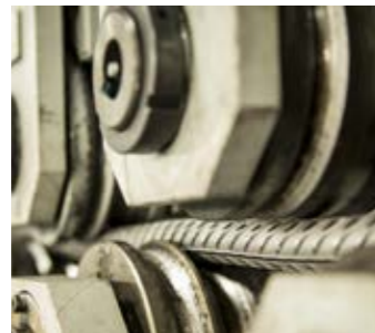
Straightening Rebar coils are straightened before cutting to lengths to remove tension in the material.
