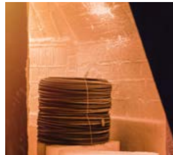
Annealing The rotary annealing furnace softens the rod to increase its ductility for further processing.
