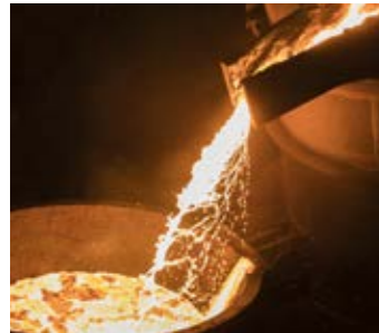
Melting shop Consistently produced high quality semis are made at SMACC in 130-tonne melts.
