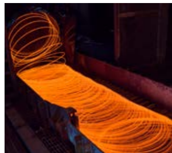
Coil forming Wire rod of up to 18 mm is coiled on a laying head.
