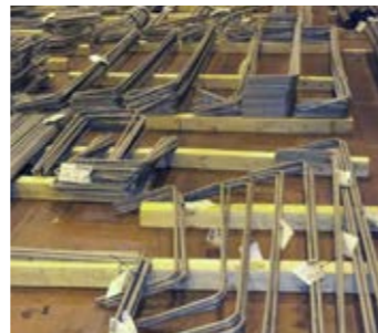
Packing Rebar shapes and lengths are carefully packed before delivery to their final destination.
