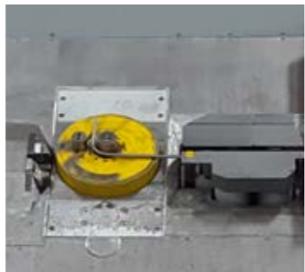
Shape bending Rebar can be bent to a number of shapes according to customer specifications.
