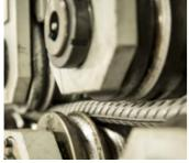
Straightening straightened before cutting to lengths to remove tension in the material.
