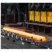
Reheating furnace Accurately controlled, two-stage reheating minimizes surface scaling.
