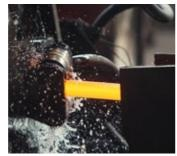
A highly responsive digital control system tracks the rod through the mill to ensure quality.
