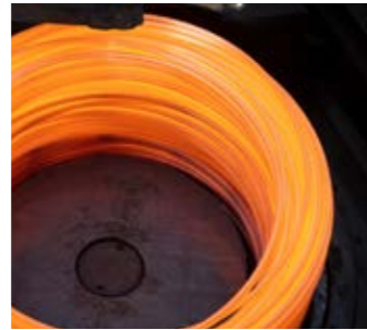
Hot rolling into wire rod Rod coil feedstock is used for bar production at Sheffield Stainless Bar.
