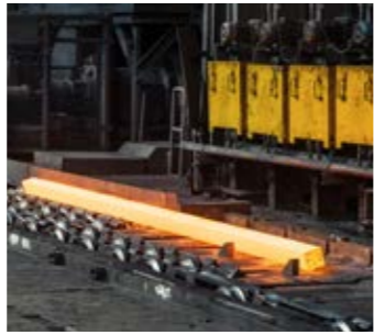
Preheating Billets are reheated before rolling into wire rod.
