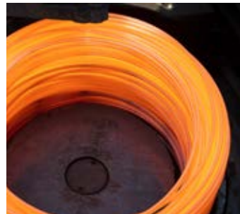
Coil forming Wire rod of up to 10 mm is coiled on a laying head. Rod in larger diameters is coiled in garret coilers.
