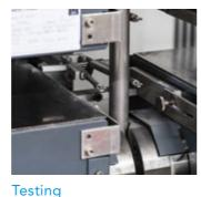
Samples from production stages are tested for surface defects, grain size, and tensile strength.
