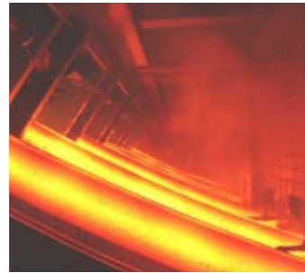
Billet casting We use a combination casting machine for slab, bloom or six-strand billet casting machine.
