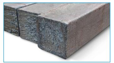
Continuously cast billets
