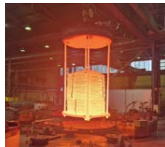
Annealing The annealing furnace softens the rod to increase its ductility for further processing.
