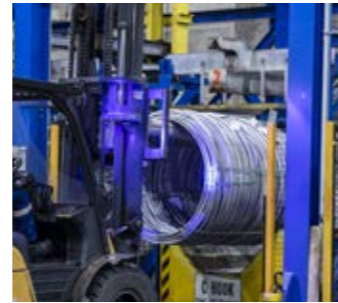
Coil pre-dipping The surface of the bar is coated with a drawing lubricant to aid cold drawing.
