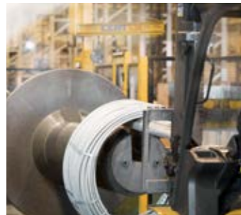
Preparation for cold drawing Rod coils are moved from the pre-dipping station to the cold drawing line.
