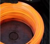
Hot rolling into wire rod Rod coil feedstock is used for bar production at Sheffield Stainless Bar.
