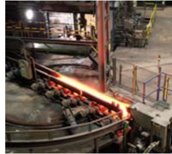
Reheating furnace Accurately controlled, two-stage reheating minimizes surface scaling.
