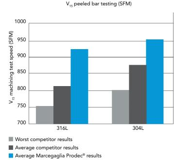
Testing done with  $Prodec^{\circ}$  and 7 European competitors' bars with improved machinability in grades 316L and 304L. The tool used for testing was a cemented carbide insert.
