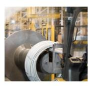
Preparation for cold drawing Rod coils are moved from the pre-dipping station to the cold drawing line.
