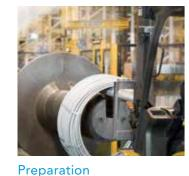
for cold drawing Rod coils are moved from the pre-dipping station to the cold drawing line.
