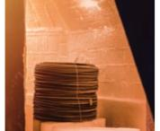
Annealing The rotary annealing furnace softens the rod to increase its ductility for further processing.
