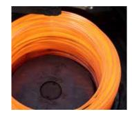
Wire rod coiling Wire rod of up to 10 mm is Rebar coils are coiled on a laying a head. Rod in larger diameters is coiled in garrett coilers.
