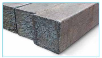
Continuously cast billets
