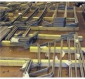
Packing Rebar shapes and lengths are carefully packed before delivery to their final destination.
