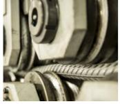
straightened before cutting to lengths to remove tension in the material.
