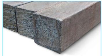
Continuously cast billets
