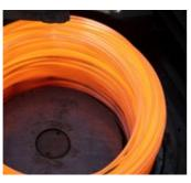
Hot rolling into wire rod Rod coil feedstock is used for bar production at Sheffield Stainless Bar.
