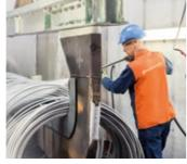
Pickling Scale is removed from the hot rolled surface using salt bath and acid treatment.
