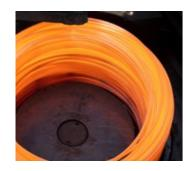
Wire rod coiling Wire rod of up to 10 mm is Rebar coils are coiled on a laying a head. Rod in larger diameters is coiled in garrett coilers.
