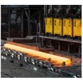
Preheating Billets are reheated before rolling into wire rod.
